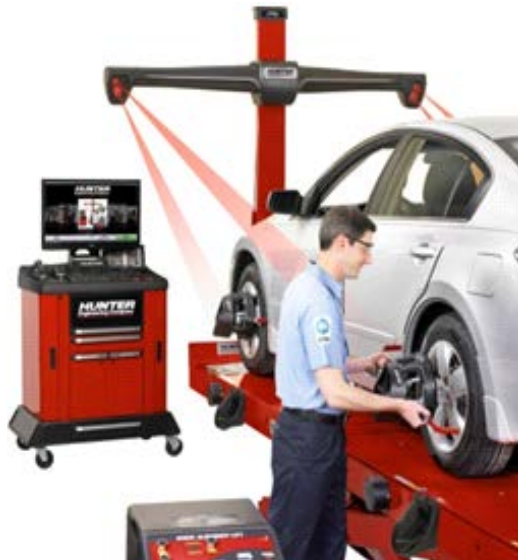
Figure 10. Computerized camber adjustment system with four high-resolution cameras
