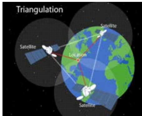
Figure 4. GPS triangulation method – the tracked object is in the intersection of a sphere
